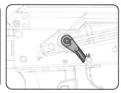
FULL AUTOMATIC MODE The gun will fire automatically while the trigger remains pulled.
